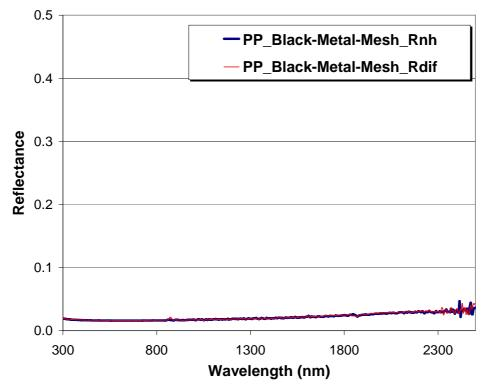
Figure 3. Total near-normal hemispherical and near-normal-diffuse spectral reflectance (Glazing (F) and Room (B) Sides) of Nysan Shading Systems sample S01 Superscreen 300 White Pearl.
