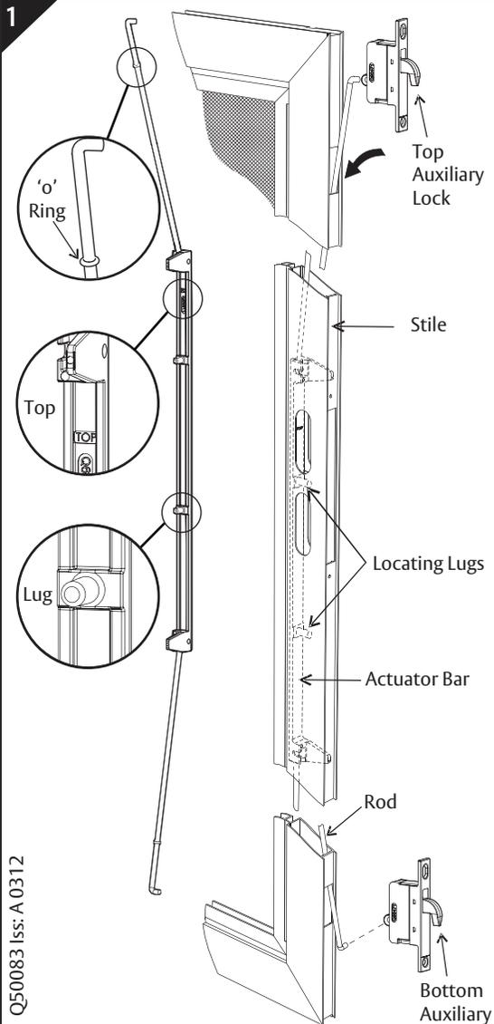
**Fitting the Actuator Bar and Auxiliary Locks**
