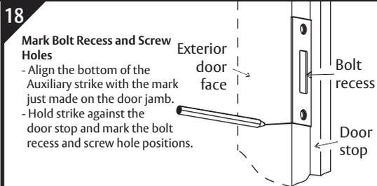
**Mark Bolt Recess and Screw Holes**
