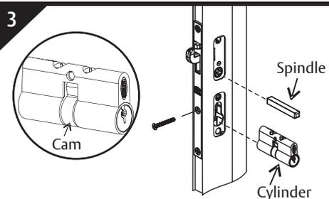
**Fitting Cylinder & Spindle**
