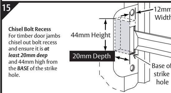
**Chisel Bolt Recess**
