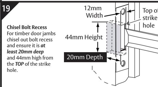
**Chisel Bolt Recess**
