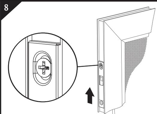
**Fixing Screw to Top and Bottom Auxiliary Locks**
