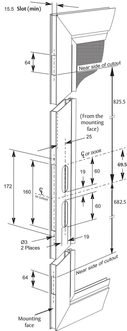
Both sides of the door section must be cut to the dimensions given. Start with the centre of door (**CL OF DOOR**) then measure **69.5mm BELOW** and mark the (**CL OF CUTOUT**).
