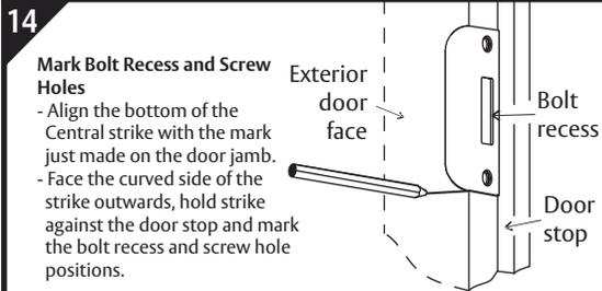
**Mark Bolt Recess and Screw Holes**
