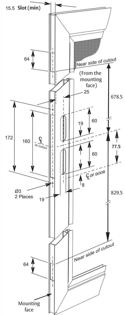
Both sides of the door section must be cut to the dimensions given. Start with the centre of door (**CL OF DOOR**) then measure **77.5mm ABOVE** and mark the (**CL OF CUTOUT**).
